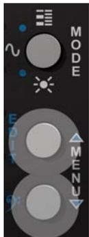
2. To step through the parameters of each device, press either of the two "Menu" buttons below the "Mode" button.
