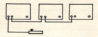
The foot switch must <u>always</u> be plugged into the jack on the left, as your looking at the unit directly from the rear. A patch cord (regular guitar cord) then runs from this unit into the left jack of the next and so on. The single foot switch will now control all of the SENSORS whose OFF-ON switch is in the ON position.
